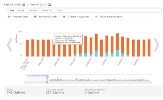
This leak – if it had been uncorrected for the entire billing quarter—would have added \$1,015 to the water bill that quarter. The property owner found a leaking toilet, repaired the leak, and avoided the high bill.
